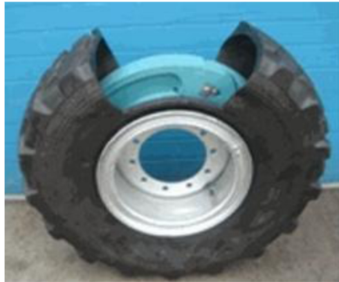
Fig. 7. The „Run flat” system [7]
