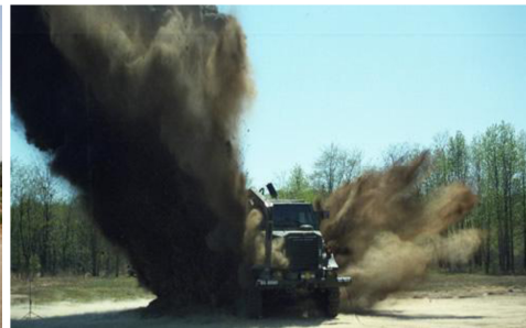
Fig. 6. Explosion of an explosive device under the vehicle Buffalo [6]
