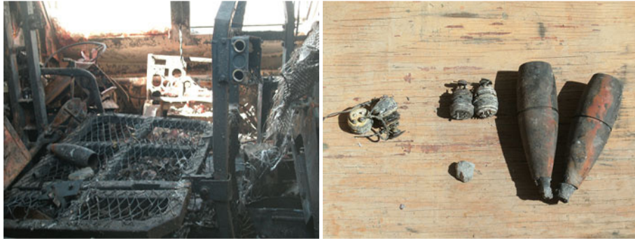
Fig. 7. Interior view of the MRAP vehicle after the fire (left) and unexploded shell bodies from M768 cartridges (right)
