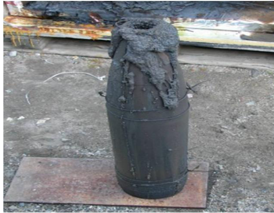
Fig. 6. Slow cook-off result of an IMX-101 filled M795
