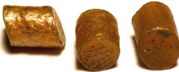
Fig. 2. Propellant grains with copper condensed on surface
