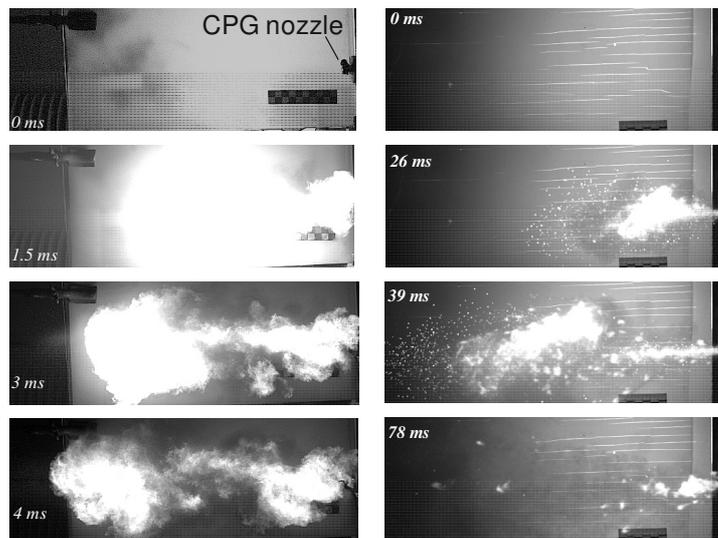
Fig. 4. Comparison of ignition phase (left – plasma, right – black powder)
