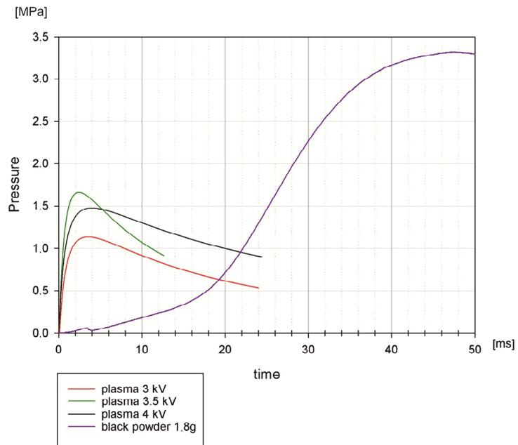
Fig. 5. Initial vessel pressurization
