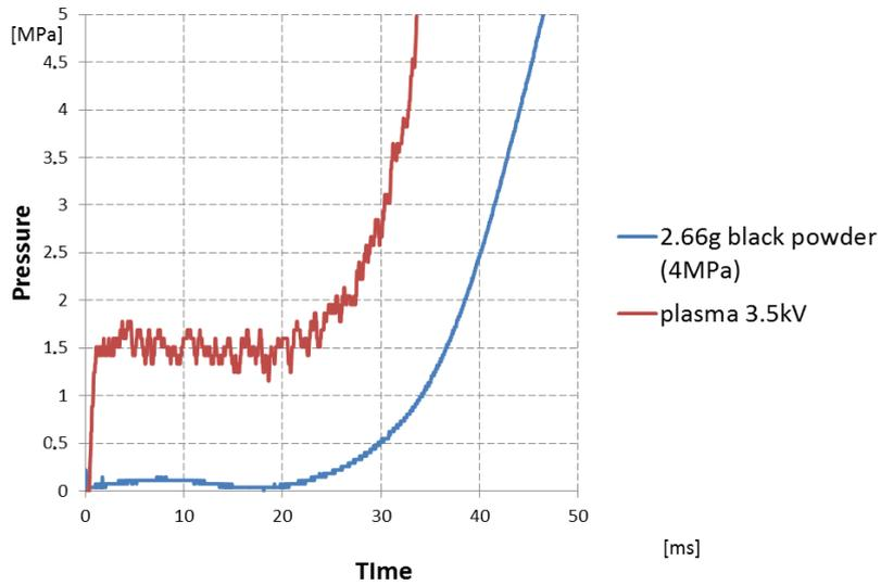
Fig. 6. Pressure graph for different types of ignition
