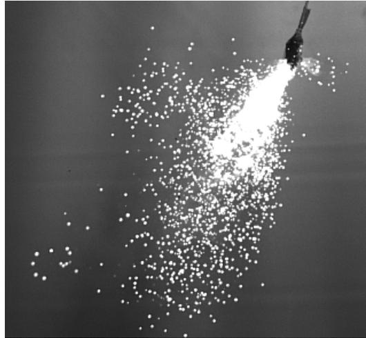
Fig. 1. Exemplary picture of black powder ignition process (visible hot solid particles)
