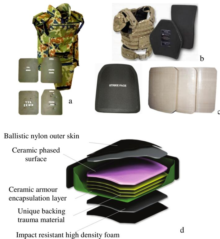
Fig. 1. Hard ballistic plates used for higher protection levels (e.g. K3÷K5 according to Polish Standard PN-V-87000:2011) in modern body armours: a – steel plates [1]; b – ceramic plates [2]; c – UHMWPE plates [3]; d – layered armour [4]
