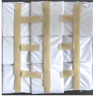
Fig. 2. Modular interlayer used for lower protection levels (K2 according to Polish Standard PN-V-87000:1999; K1 according to Polish Standard PN-V-87000:2011) in the *Smart Armour* project
