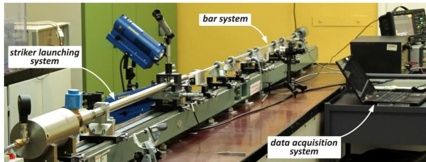
Fig. 3. The PMMA split Hopkinson pressure bar set-up
