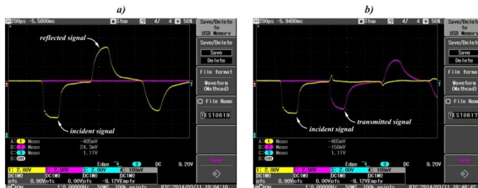
Fig. 4. The raw viscoelastic wave signals measured by the strain gages:
