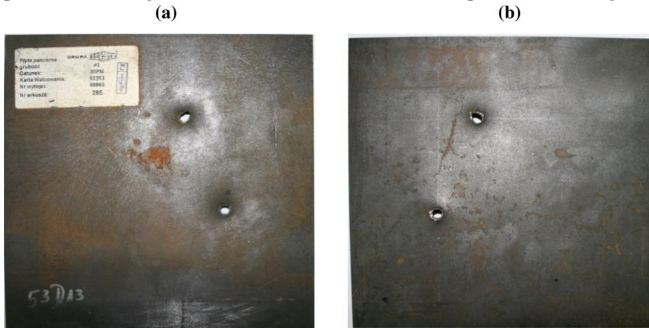
Fig. 7. 30PM steel plates of 3 mm thickness after normal perforation tests (a) impact surface (b) rear surface
