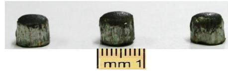
Fig. 12. Resulting plugs after shots of 6.4 mm 30PM steel plates
