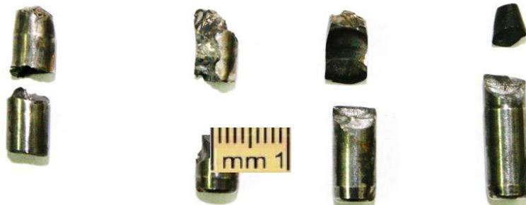
Fig. 24. Bullet core after 60° oblique perforation tests
