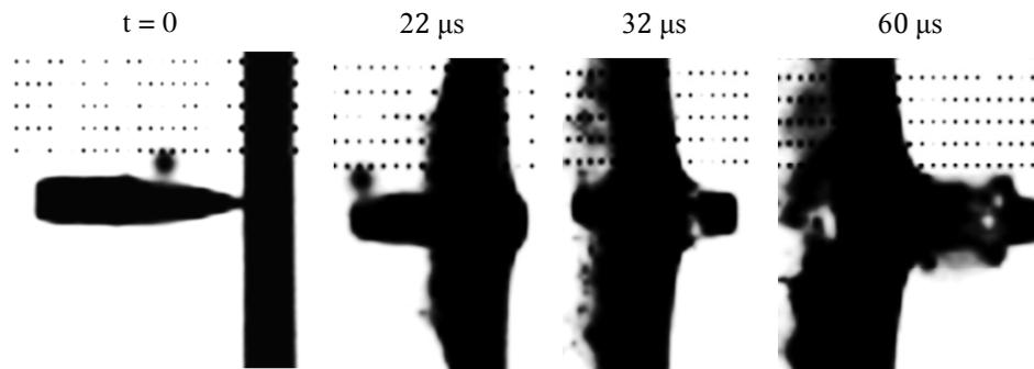
Fig. 13. High speed camera images of perforation tests of 6 mm thickness 30PM steel plates
