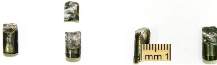
Fig. 21. Bullet core after 50° oblique perforation tests
