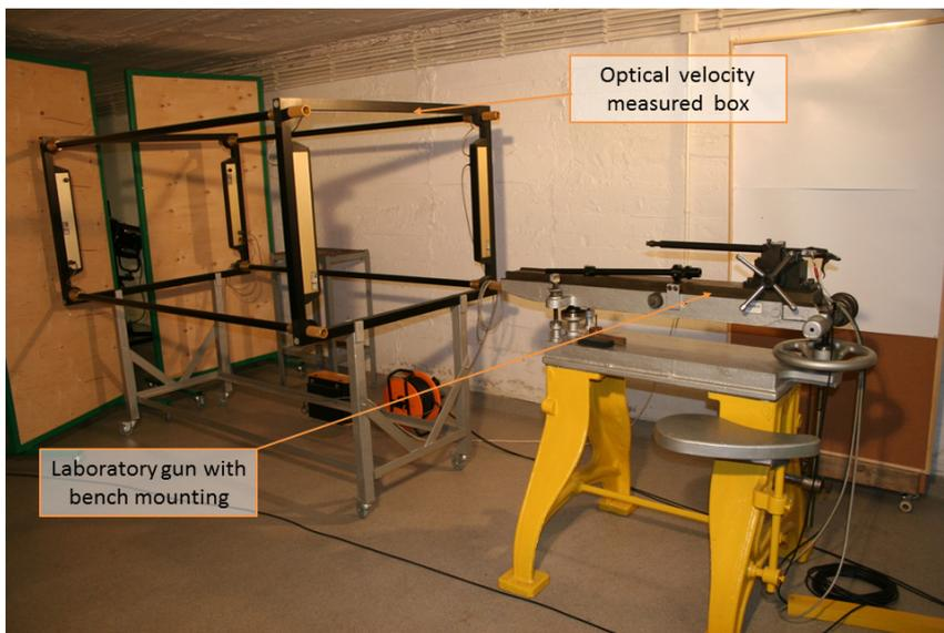
Fig. 4. Laboratory gun and optical velocity measurement system
