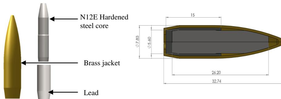
Fig. 2. Schematic drawing geometry of 7.62 mm AP bullet
