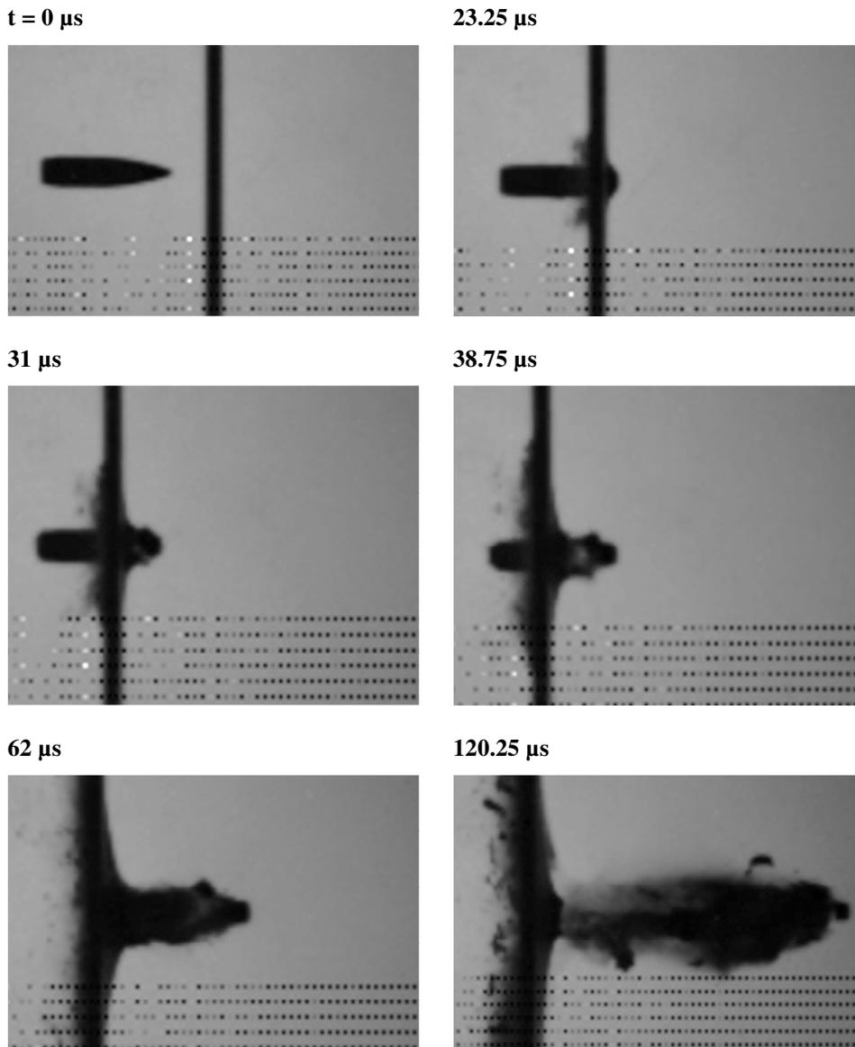
Fig. 8. High speed camera images of perforation tests of 3 mm thickness 30PM steel plates
