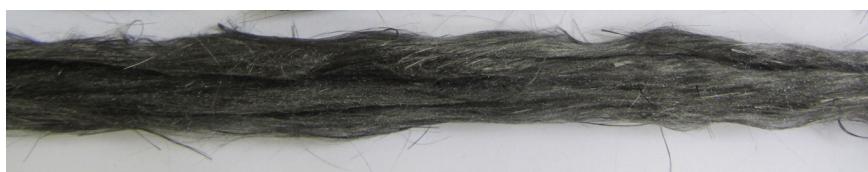
Figure 5. Draw frame sliver manufactured from 80 mm staple CF.
