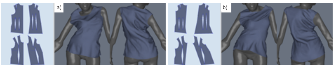
Figure 6. Pattern alteration proces with modifications of darts (a) and side lines (b).
