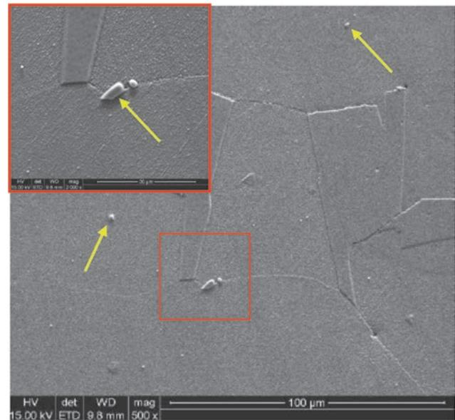
Fig. 4. Microstructure of 800HT alloy in its delivery condition; arrows indicate TiX primary precipitates, SEM
