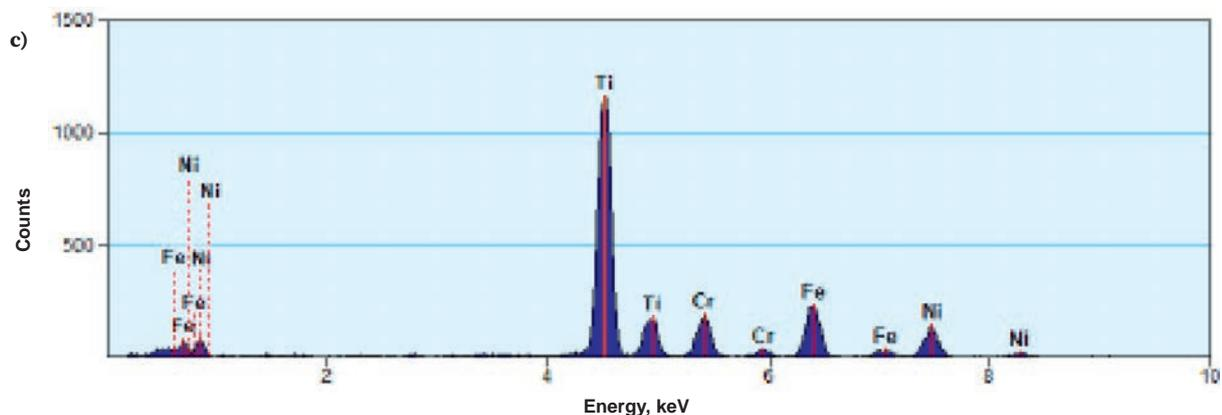
Fig. 5. TiX precipitate in 800HT alloy in its delivery condition: a) dark field; b) resolved diffraction; c) EDS spectrum
