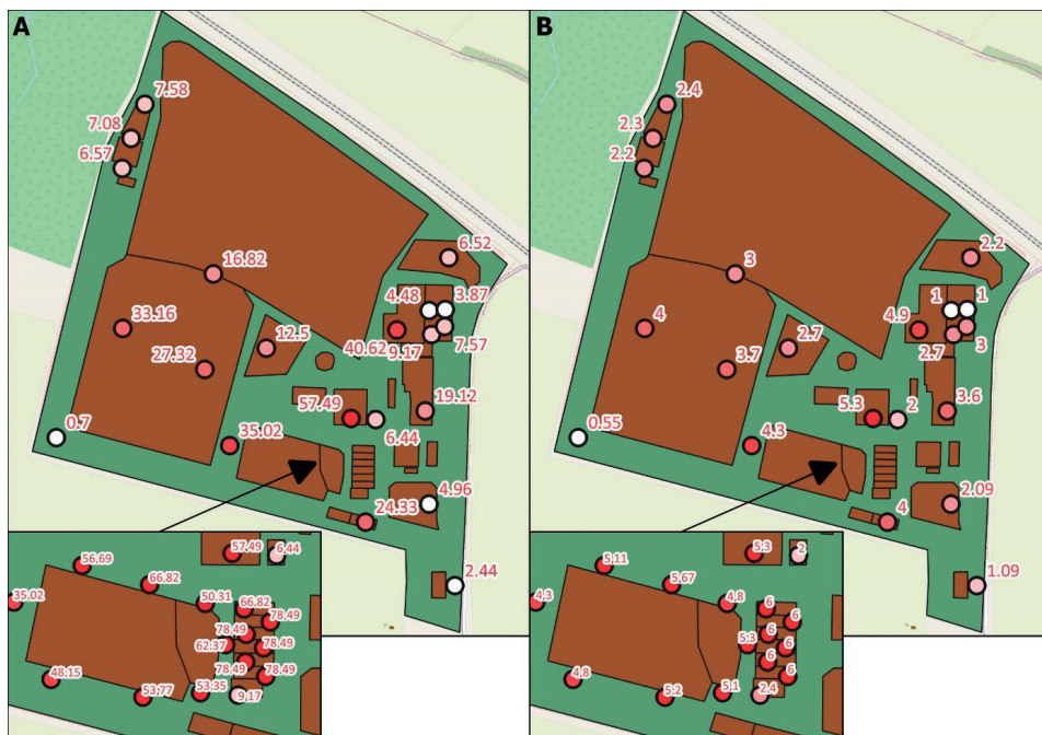
Figure 4. Average odour concentration (A) and average odour intensity (B) for each measuring point located at Facility, based on a 11-month measuring period
