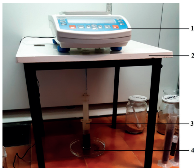
Figure 2. Test stand for the capillary seeping method: 1 – laboratory scale, 2 – anti-vibration table, 3 – measuring container with sorbent, 4 – weighing dish with sorbate
