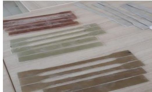
Fig. 2. Tensile and flexural tests of composite specimens
