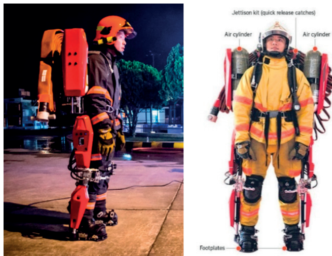
Figure 5. The Auberon Pneumatic Exoskeleton is designed to provide relief for firefighters carrying up to 40 kg of firefighting equipment up the stairs of burning high-rise buildings
