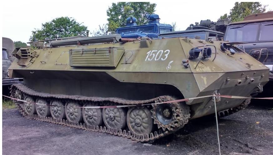
**Fig. 14.** MT-LBu carrier in the MP-21 command-staff version
